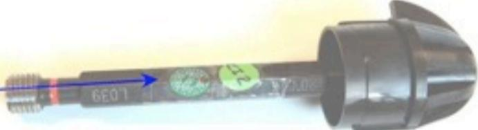
(32) PROVA FILETTATURA M.12 X 1.25 CON TAMPONE P. NP. CODICE CI2
